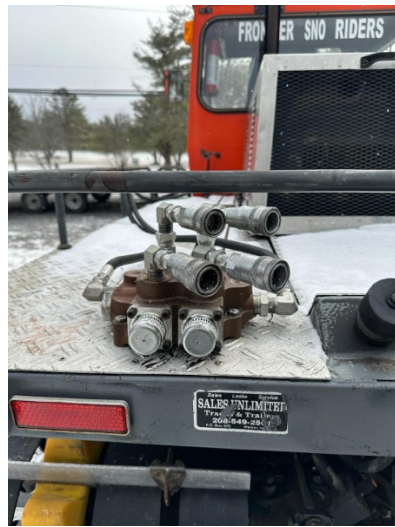
The hydraulic fitting upgrades, on the left is the old position, the right side shows the new elevated couplers.
